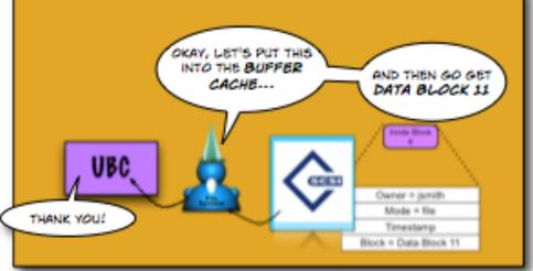
The data is put into the Unified Buffer Cache (i.e., specifically an Inode cache)
