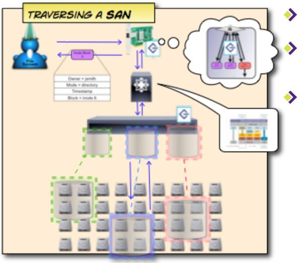
SANs insert SCSI communication networks Permit consolidation of storage for multiple hosts over a storage network Each host controls (i.e., "owns" its assigned storage)
