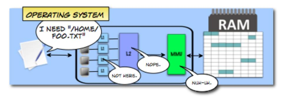
Operating System checks main memory (and associated caches) first
