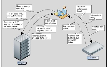
A **Storage Management Standard** provides a common language for these messages between a storage management application and the instrumentation for storage systems. SMI-S is unique in providing a standard that allow multiple storage applications to manage a variety of storage systems from a variety of vendors.
