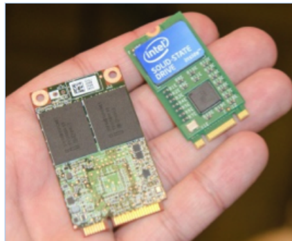
Figure 1. mSATA (left) and M.2 (right) Form Factors
