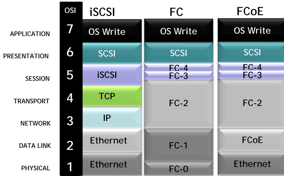
Fibre Channel is a layered protocol. It consists of 5 layers, namely:
