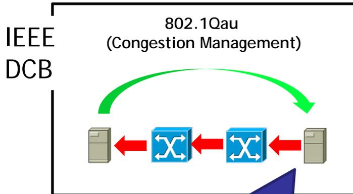
End-to-End Communication between end-points. Tells the end-point to BACK OFF!
