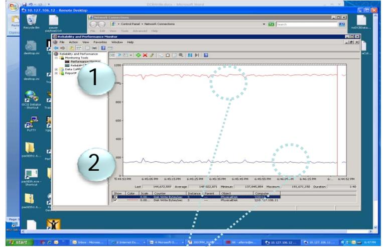
Unbalanced iSCSI throughput (1100MB/s, 100MB/s)
