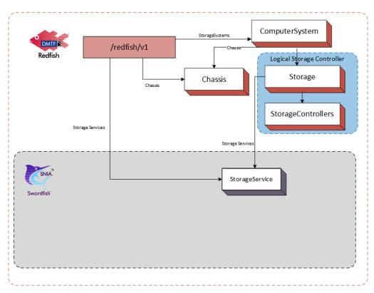
Figure 6: Logical Subsystem in Integrated Service Configuration
