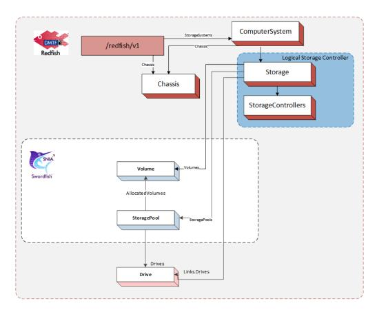
Figure 5: Swordfish Integrated Configuration Example
