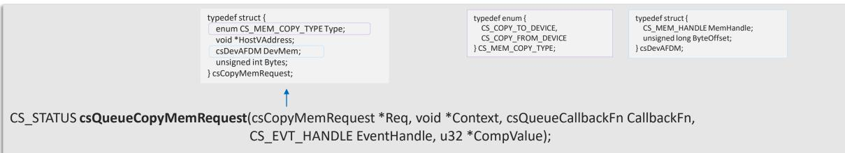
Transfer data between Host memory and allocated Device Memory
