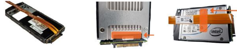
Figure 3. Quarch Interposer Board & Ribbon Cable
