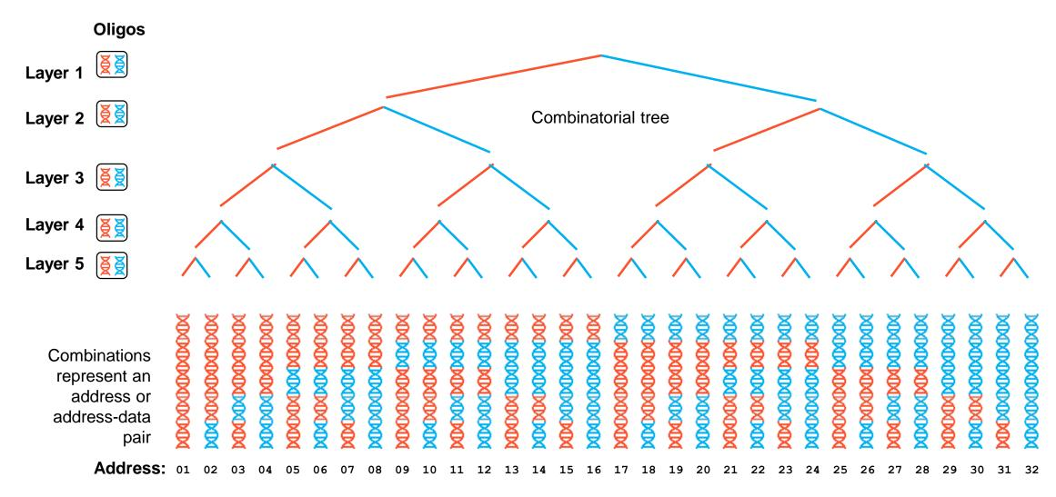
Scales exponentially: L layers of N components enables N<sup>L</sup> bits of information with only LN oligos
