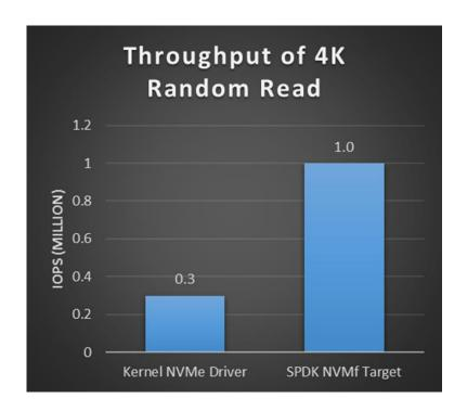
Throughput of NVMf with polling user driver can reach ~1.0M IOPS, with only 1 CPU cores utilized
