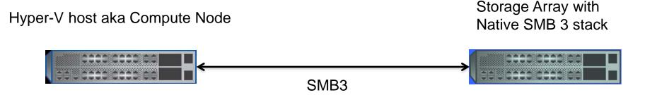
When Storage array offers a Native SMB 3 interface, you end up with a minimum of just 2 rack mount units !
