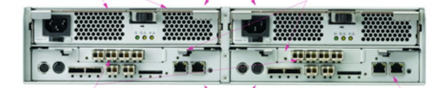
Fibre Channel front-end connectivity for multi-pathing
