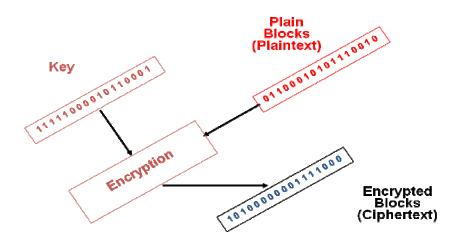
Decryption is therefore the reverse process, in which two inputs, namely ciphertext and a key), produces a single output, namely plaintext.
