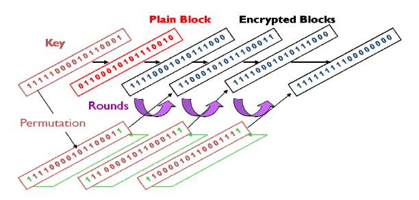
Each process is known as a round, and the cryptographic "mode" defines how output of one round becomes input of another.
