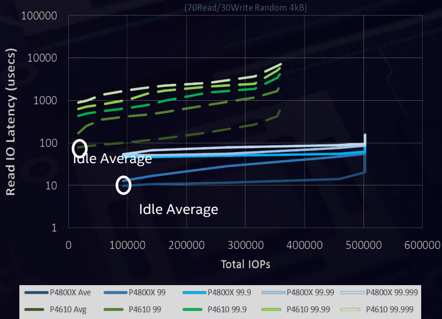
Latency vs. Load: NAND SSD vs. Intel® Optane™ SSD 2 (Intel® DC P4610 3.2TB vs. Intel® Optane™ SSD DC P4800x 375GB)
