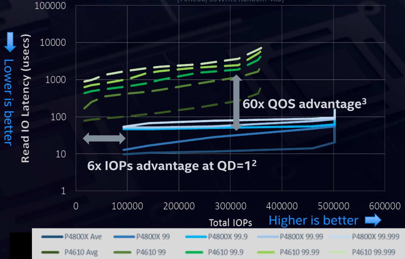
Latency vs. Load: NAND SSD vs. Intel® Optane™ DC SSD 1 (Intel® DC P4610 3.2TB vs. Intel® Optane™ SSD DC P4800x 375GB) (70Read/30Write Random 4kB)
