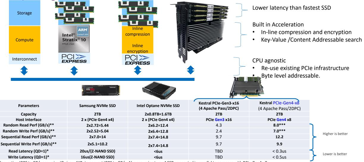
\*\* Converting IOPS to GB/s assuming IO size = 4KB. to convert IOPS to GB/s. Also assuming two x4 SSD connected in parallel to compare with PCIe-Gen4-x8.
