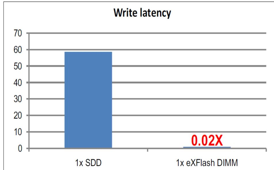
Figure 15 eXFlash DIMM versus SSD: write latency
