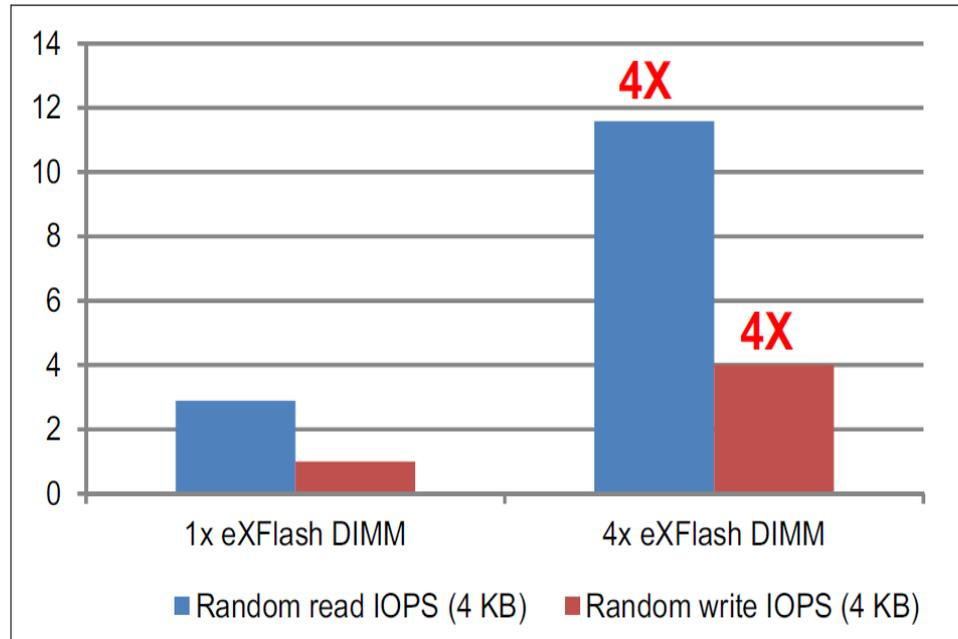
Figure 12 eXFlash DIMM scalability
