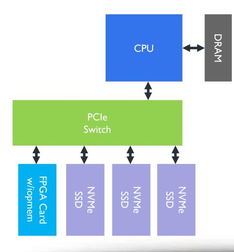
Use FPGA with exposed BAR as iopmem device.
