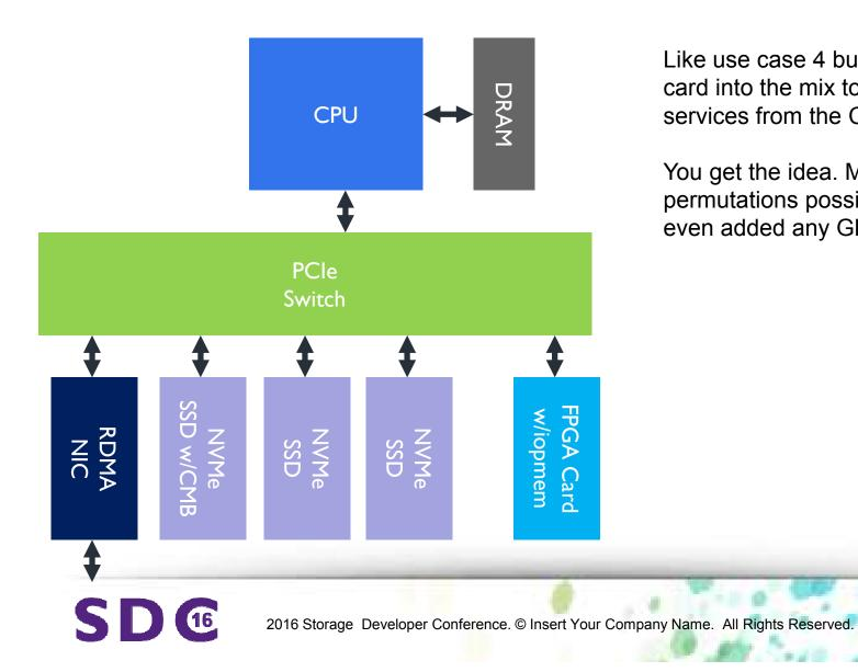
Like use case 4 but add the FPGA card into the mix to offload storage services from the CPU.
