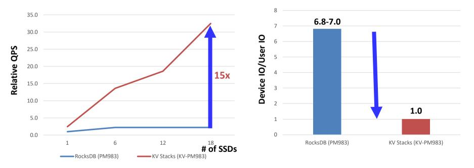
Relative performance to the maximum aggregate RocksDB random Put QPS for 1 SSD with a default configuration for 1 PM983 SSD in a clean state. System: Ukume 16.04.2 LTS, , Ext4, RAIDO for block SSDs, Actual CPU utilization could be 70-90% at CPU saturation point. Workoad: 100% put 6 byte201/7 StoragemDevielopersConference.r@cksDB v. SAMS UNCalues, 24IR ights: Reserved with 4 client up ads, 50GB/Instance or 1.2TB Data is used
