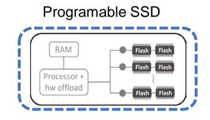
Trusted domain for secure computation; cleartext not allowed to egress this boundary
