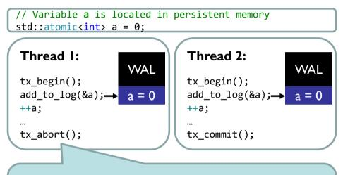
Incorrect value of the counter is restored from undo log if thread 1 aborts transaction while thread 2 successfully commits its changes.
