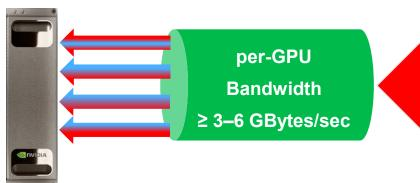
per-GPU data access up to ~11 GBytes/sec (100-gbit/s networks) or ~22 Gbytes/sec (200-gbit/s IB)
