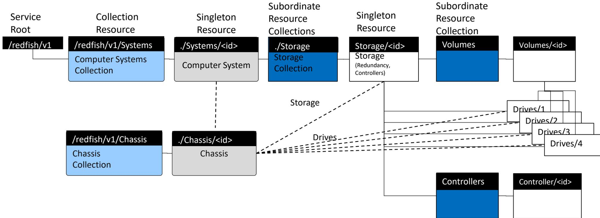
Note that the Volumes are in Collections off of the Storage resource, drives are in arrays off of the storage resource and optionally the Chassis.
