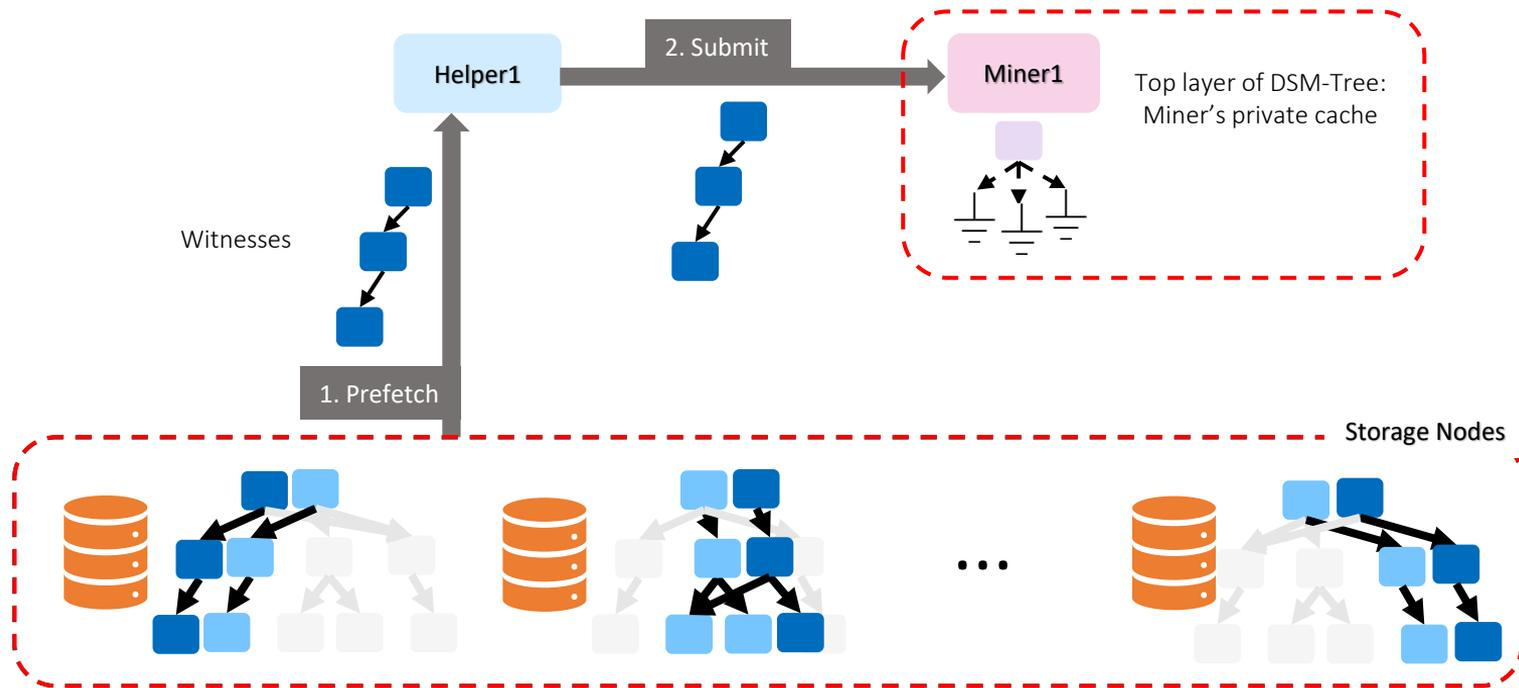
The DSM-Tree layers collaborate with each other to reduce network traffic
