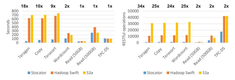
As compared with the object storage connectors of Hadoop 2.7.3 run with their default parameters with Spark 2.0.1 See https://arxiv.org/abs/1709.01812
