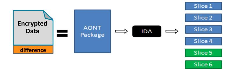
Without a threshold number of slices, cannot calculate hash and thus cannot separate key out of difference which is XOR of key and hash
