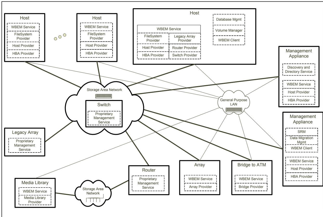
**Figure 7 - Example Client Server Distribution in a SAN**
