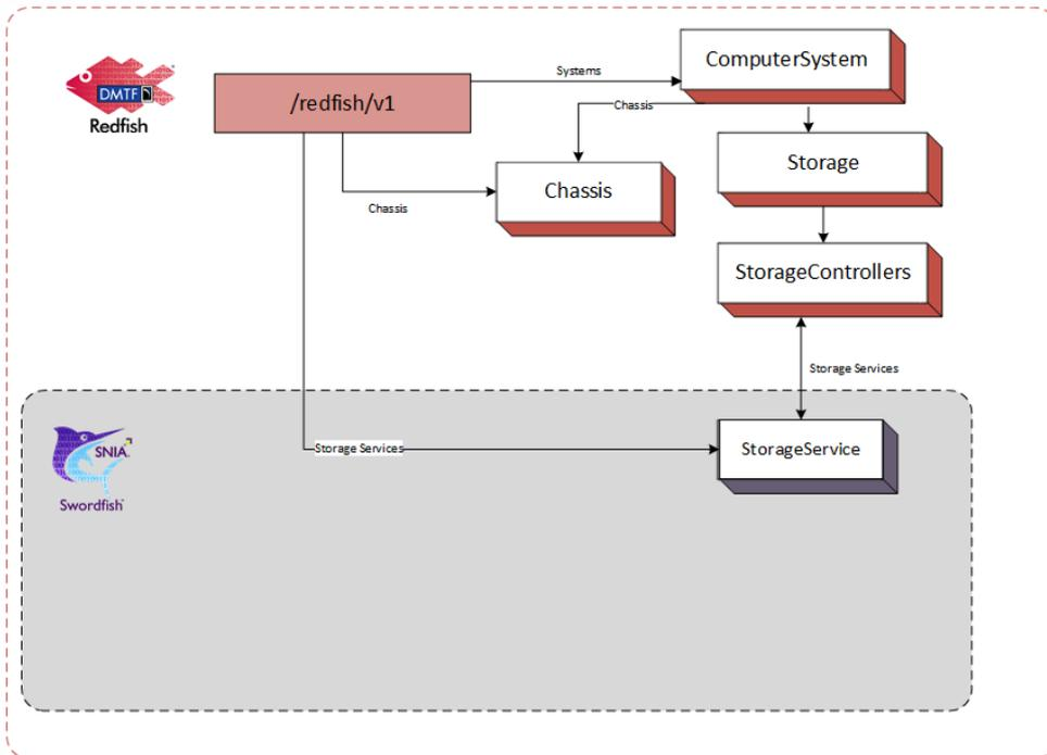
This configuration works well when the storage service is hosted by a storage resource within a computer system. An example of a Storage Service for an integrated service configuration is shown below.
