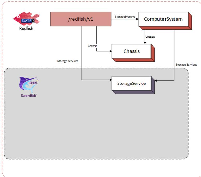
This configuration works well when the storage system hosts the storage service directly. An example of a Storage Service for a hosted service configuration is shown below.
