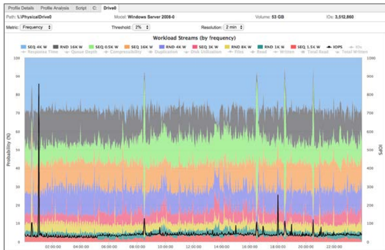
IO Stream Map: 24-hour Block IO Level (Drive0) Capture showing IOPS & IO Streams
