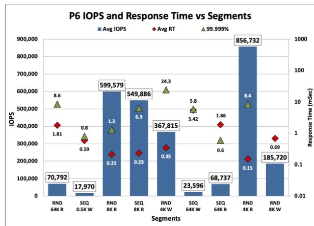
**Figure 35 – Individual Streams Test: IOPS & RTs v Segments.** Individual IO Streams run to Steady State
