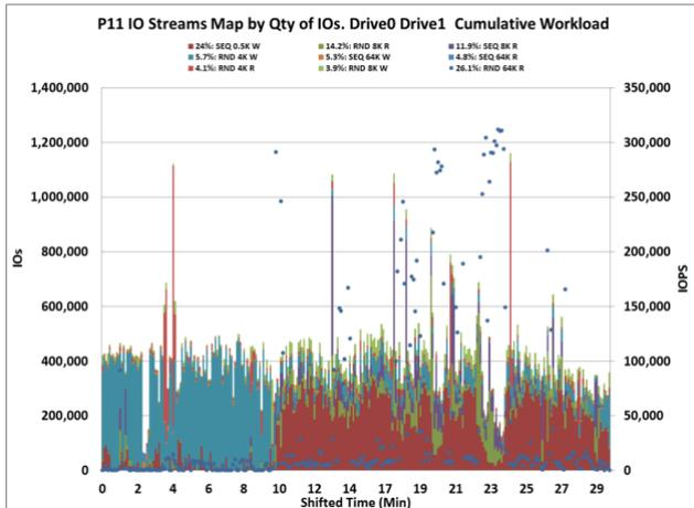
**Figure 30 – IO Stream Map & IOs.** Sequence of IO Stream Combinations, IOs & IOPS on NVMe SSD
