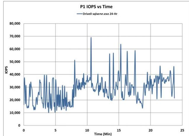
**Figure 31 – Replay Test IOPS v Time.** IOPS measured during a Replay test run on NVMe SSD
