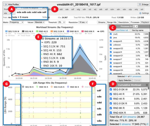
**Figure 15 – Aggregate IO Stream & LBA Maps.** See aggregate and individual storage IO and LBA Range Hits
