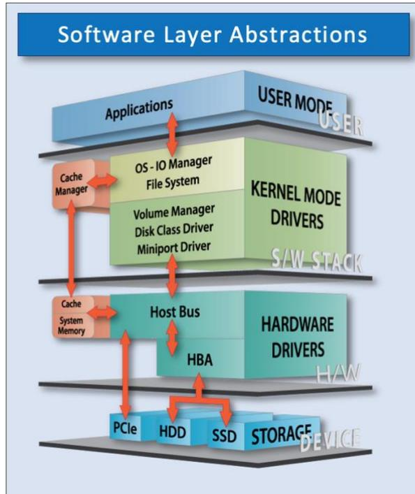
Figure 1 - SW/HW Stack. IO Streams merge, append, coalesce and split as they traverse the SW/HW Stack
