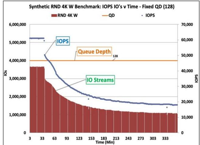
**Figure 4 – Synthetic Workloads.** Single, or few, IO Stream(s) at a fixed Demand Intensity and Duration
