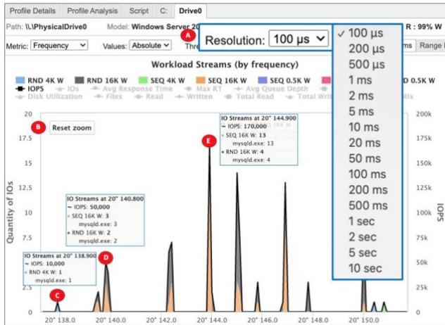
**Figure 20 – 100uS Steps.** Fine grain resolution allows observation of single or very few IO events/occurrences
