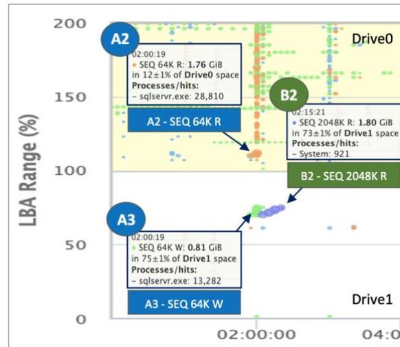
Figure 11 – LBA Hits Map. SEQ 64K R Drive0 (A2) to SEQ 64K W Drive1 (A3). SEQ 2048K Read on Drive1 (B2).
