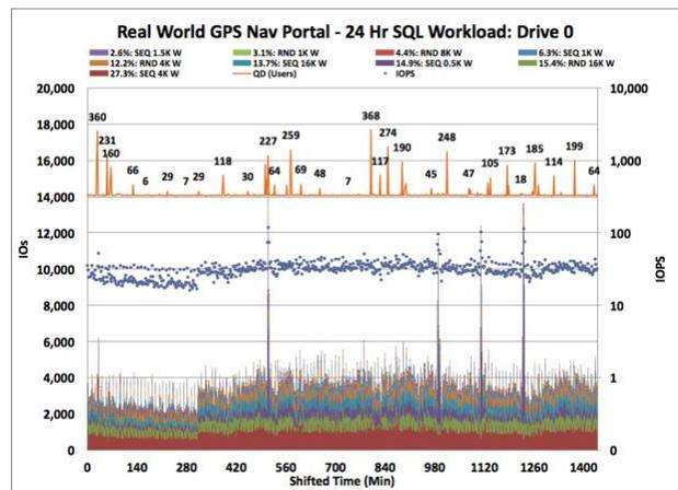
**Figure 13 – GPS Nav Portal: Storage Drive0.** 96% W; 61% RND/SEQ 4K/8K/16K; Median QD 8; Max QD 368
