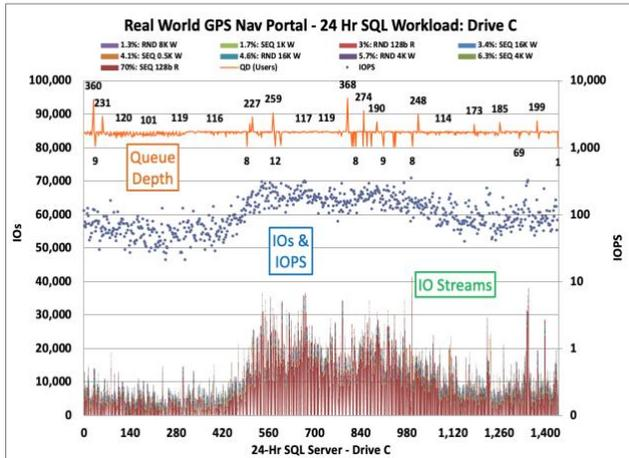
Figure 23 – GPS Nav Portal: DriveC Boot Drive
