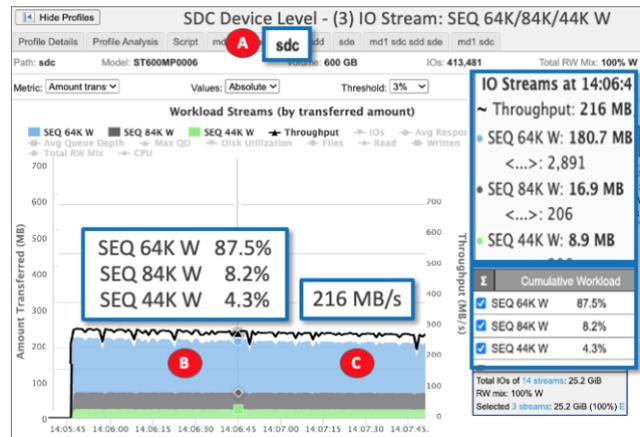
Figure 17 – IO Stream Map Device sdc. Transmuted IO Streams from RAID md1 to individual device sdc.
