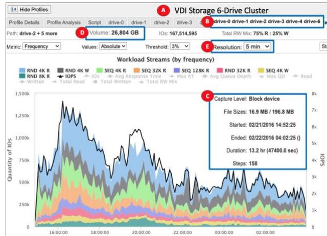
**Figure 21 – 5 min Steps.** Coarse grain resolution allows viewing of multiple/aggregate drive, long duration captures
