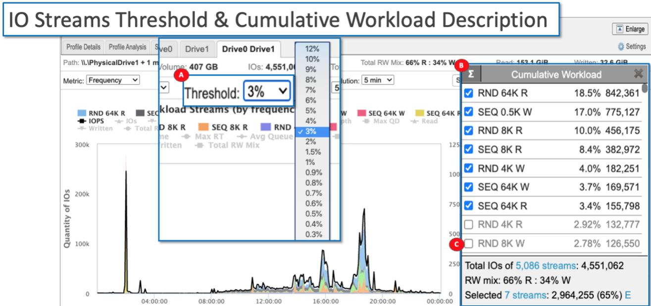
Figure 18 – Filter IO Stream Maps by IO Stream Threshold & Workload Descriptions
