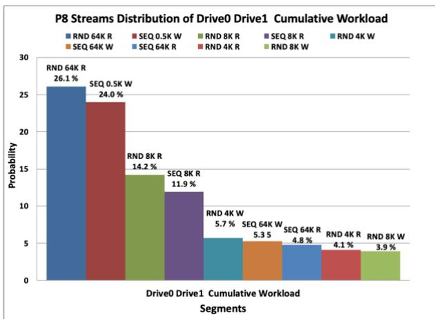
**Figure 34 –Workload Streams Distribution.** Individual IO Streams applied for each Steady State test step
