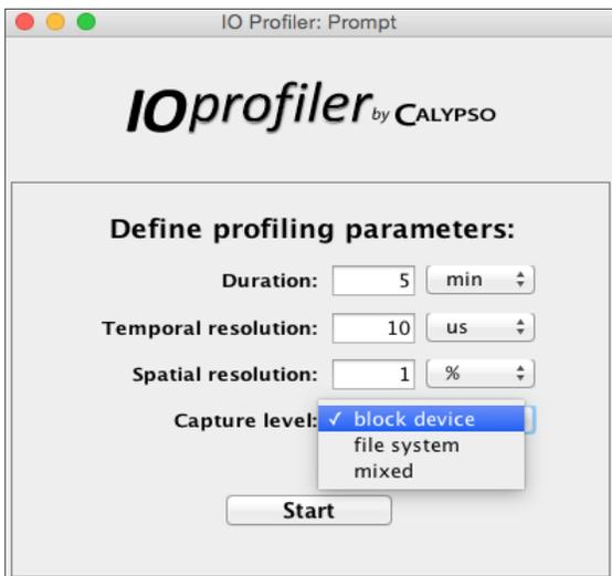
Figure 5 – IOProfiler IO Capture Tool. Set IO Capture Parameters before starting an IO Capture
