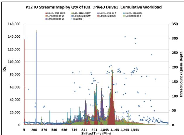
Figure 28 – Self-Test IO Stream Map & IOs. Sequence of IO Stream Combinations, IOs & QDs during IO Capture
