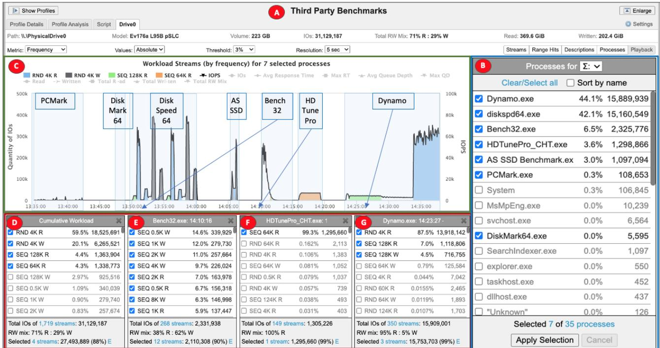
Figure 19 – Filter Applications by Process IDs
