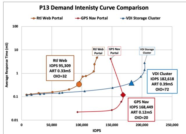
**Figure 33 – DI Curve Comparison.** “Better Performance” is at the “Lower Right Corner” of the DI OS Curve plot.
