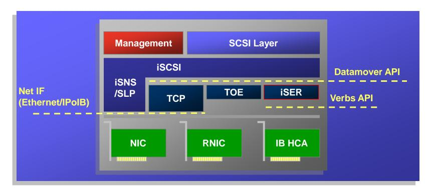
The transport layer iSER and/or iSCSI/TCP are transparent to the user. Just need a simple configurable to decide
