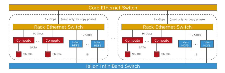
HDFS I/O ALWAYS comes through a rack-local Isilon node which collects data blocks from all other Isilon nodes across the InfiniBand fabric
