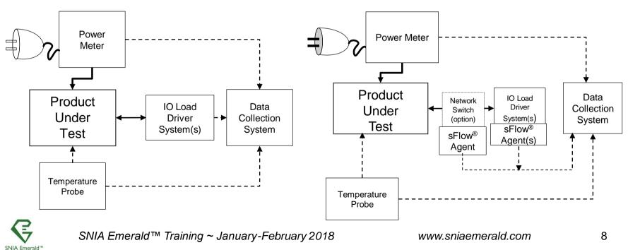
Using alternate IO measurement boundaries
