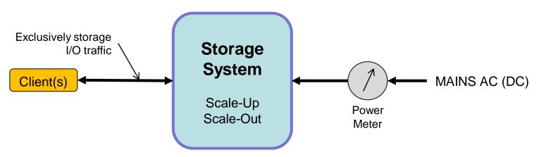
An appliance typically composed of dedicated compute, persistent storage, and interconnect functions managed by storage-oriented SW
