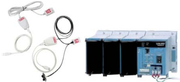
Figure 6 - Example USB Connected Remote Temperature Monitor Device (Digi Watchport®) and Yokogawa MW100 DAQ
