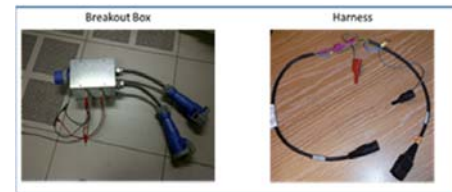
Figure 4 - Power Connection Example Using Breakout Box
