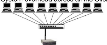
NAS Clients move the File System overhead to the NAS server
