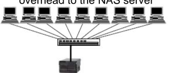
Block I/O (including iSCSI) Storage Controllers just store the I/O blocks where the Client File System requests (perhaps with Virtualizing LUN Mapping) NAS Servers centralizes the File System functions (and overhead) for all its clients into the NAS Server Plus the NAS Server still must map the resultant Blocks onto the Storage (perhaps with Virtualizing LUN Mapping)
