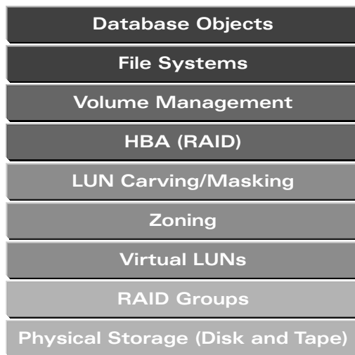
FIGURE 1-2 Typical Storage Functions Mapped to the SNIA Shared Storage Model
