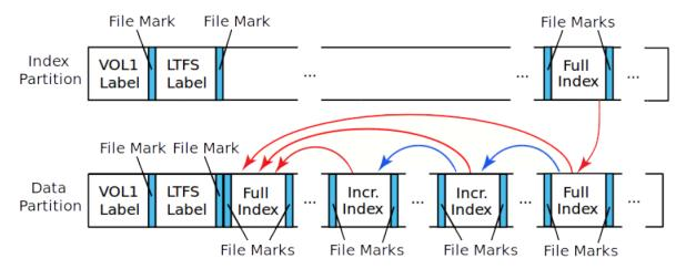
Figure 7 — Back Pointer example for Incremental Indexes
