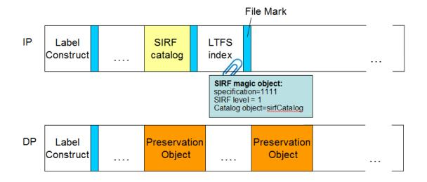
Figure 4 - SIRF Serialization for LTFS Volume
