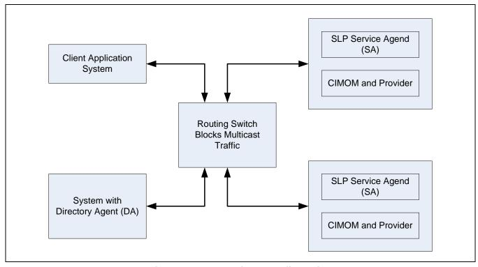
Figure 20 - No Multicast configuration
