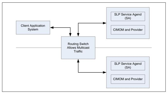
**Figure 19 - Multicast Configuration**
