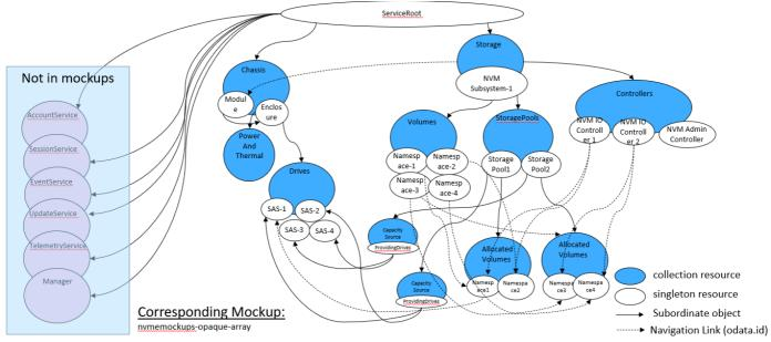
Figure 13: Sample opque system instance
