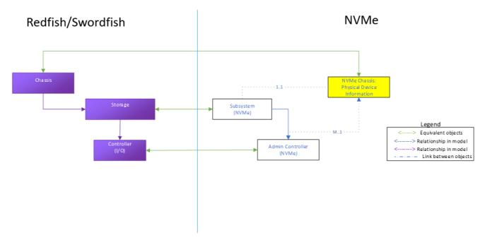
Figure 9: JBOF configuration controller object
