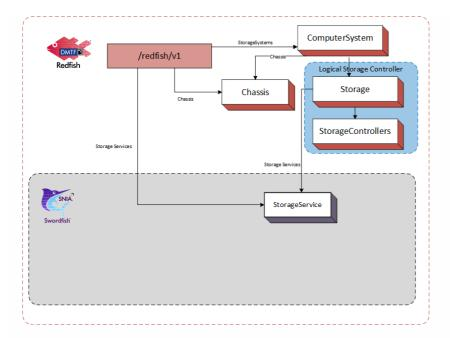
This configuration works well when the storage service is hosted by a storage resource within a computer system. An example of a Storage Service for an integrated service configuration is shown below.
