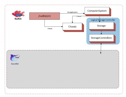
This configuration works well when the storage system can be modeled by simply instantiating a new Storage object within an existing computer system. An example of a Storage System for an integrated configuration is shown below.
