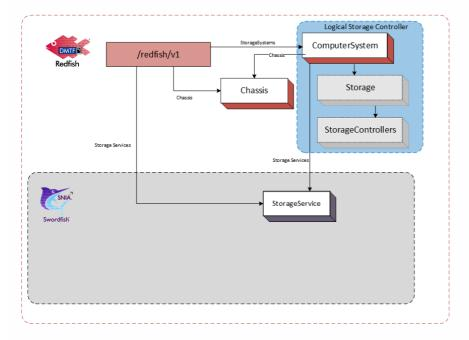
This configuration works well when the storage system hosts the storage service directly. An example of a Storage Service for a hosted service configuration is shown below.
