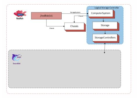
This configuration works well when the storage system needs a new ComputerSystem instance to model the logical controller. An example of a Storage System for a hosted service configuration is shown below.
