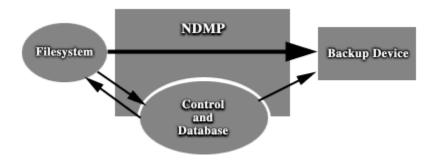
Figure 2: Common Architecture of Backup with NDMP
