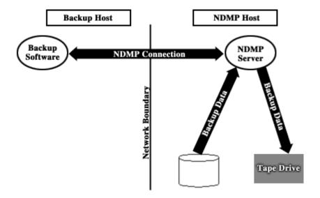
Figure 3: Simple NDMP Configuration
