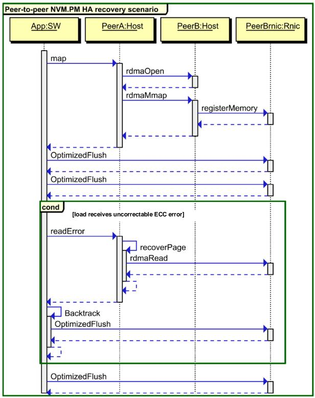
Figure 11 - Uncorrectable Error Recovery
