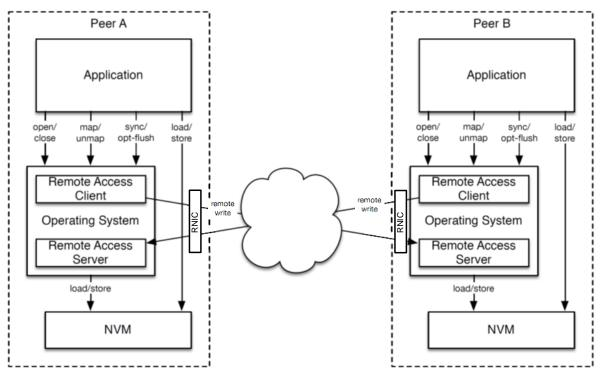
Figure 8 – NVM.PM Peer to Peer HA Replication Deployment Diagram
