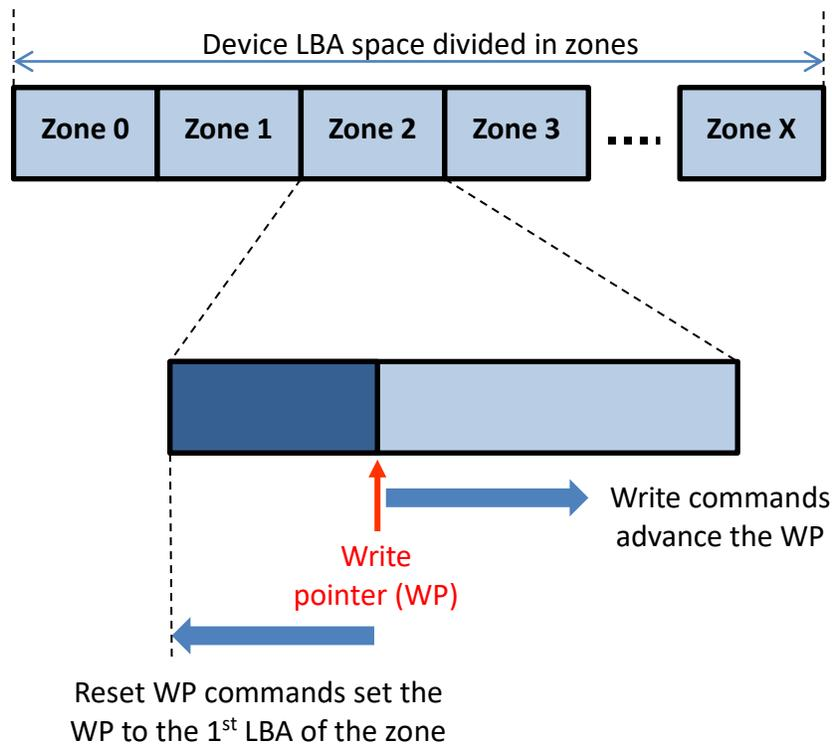
Figure 1 – Conventional device and ZNS device internal data placement
