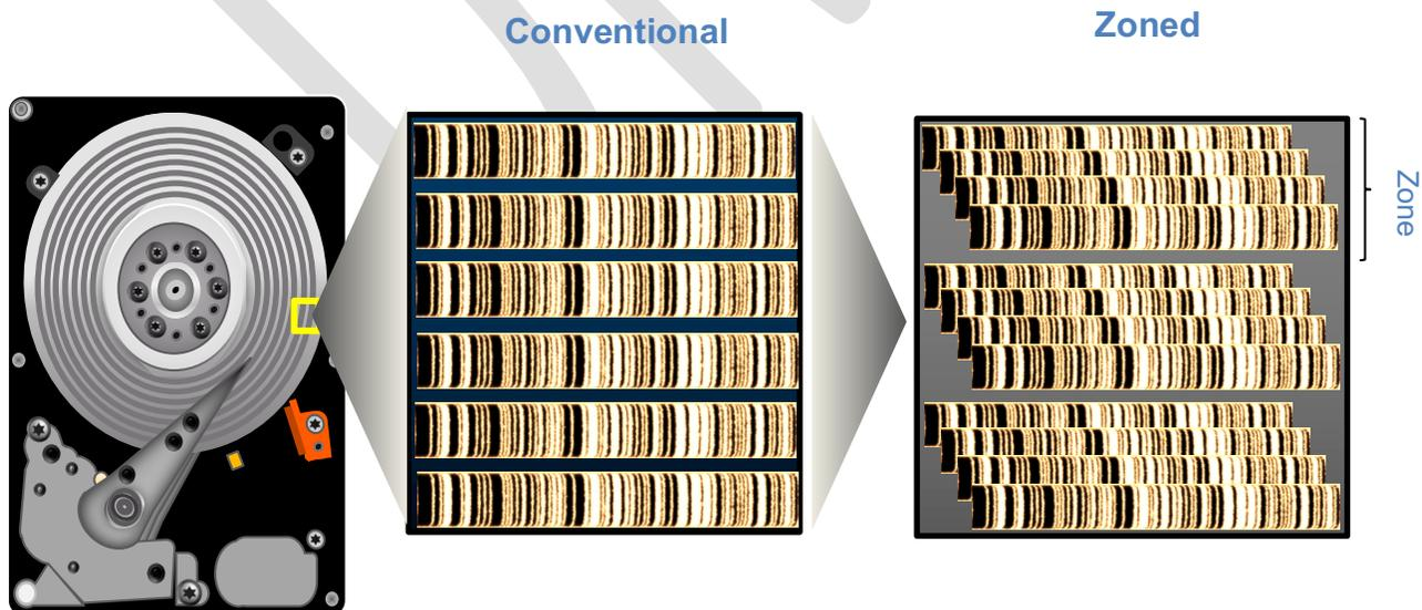
Figure 3 – Conventional device and Zoned Storage device internal data placement
