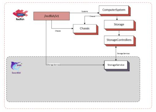
Storage resource is located in the Redfish hierarchy contained by ComputerSystems, typically running as ApplicationServers. The physical infrastructure is modeled using Redfish Chassis.
