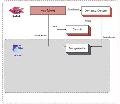
This configuration works well when the storage system hosts the storage service directly. An example of a Storage Service for a hosted service configuration is shown below.
